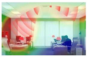
The presence sensor\* also helps direct airflow away from you for draught free comfort. While the floor sensor\* monitors temperature difference between the floor and ceiling to maintain even temperature and prevent temperature stratification in the space.
