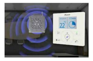
When there is nobody in the room, the presence sensor\* adjusts the set point or switches off the unit, avoiding unneccesary cooling or heating. When motion is detected the temperature is reset to its original setpoint ensuring perfect, energy efficient operation.
